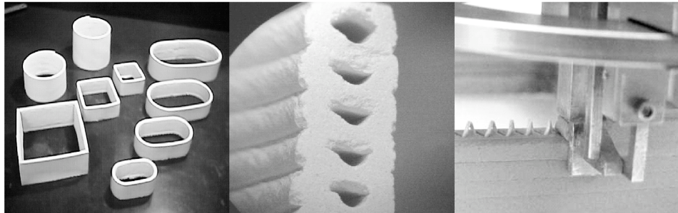
Figure 3 Demonstrations of CC constructability; (left) simple geometries, (middle) cross section of the fabricated part revealing hollow depositions, and (right) metal coil imbedding
